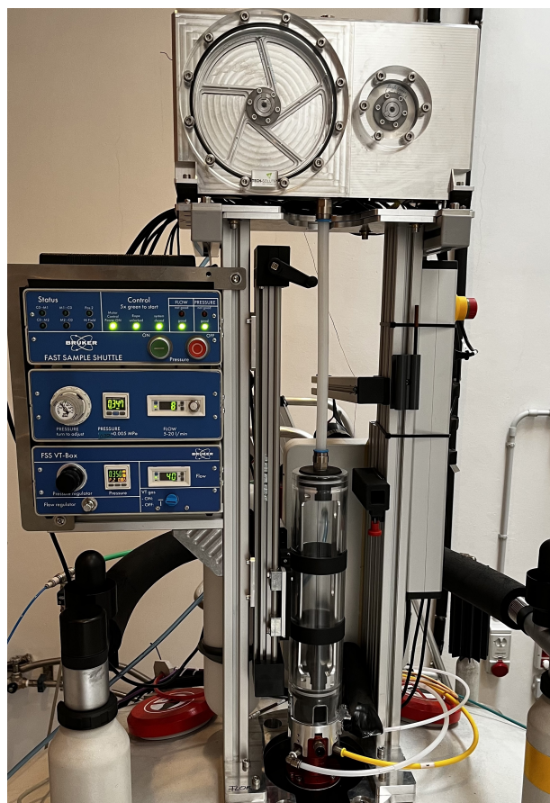
Figure 2. Photograph of the FSS installed on the 700 MHz NMR spectrometer at CERM in Florence, Italy.
