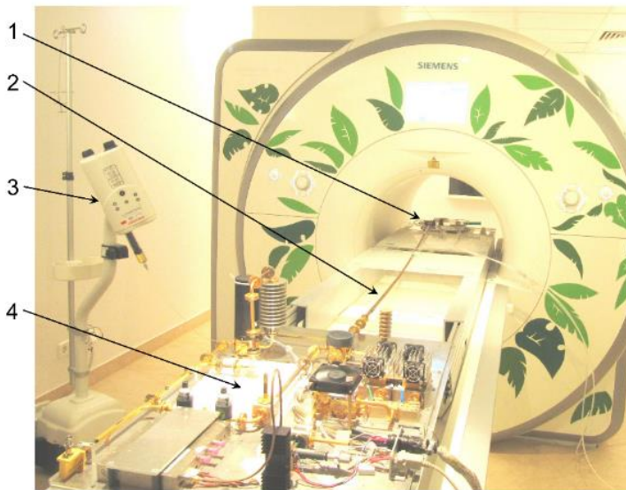
Figure 5: In-bore Overhauser DNP-MRI setup. 1- mw resonator, 2- waveguide between the mw resonator and the microwave board, 3- syringe pump, 4- microwave board.
