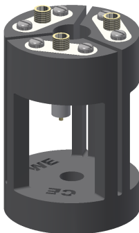
Figure 2. Cell holder consisting of the 3D-printed frame (black) and three SMA coaxial connectors (white and gold). The electrolysis cell is fixed inside the cell holder and the electrode wires are soldered to the pins of the SMA coaxial connectors.
