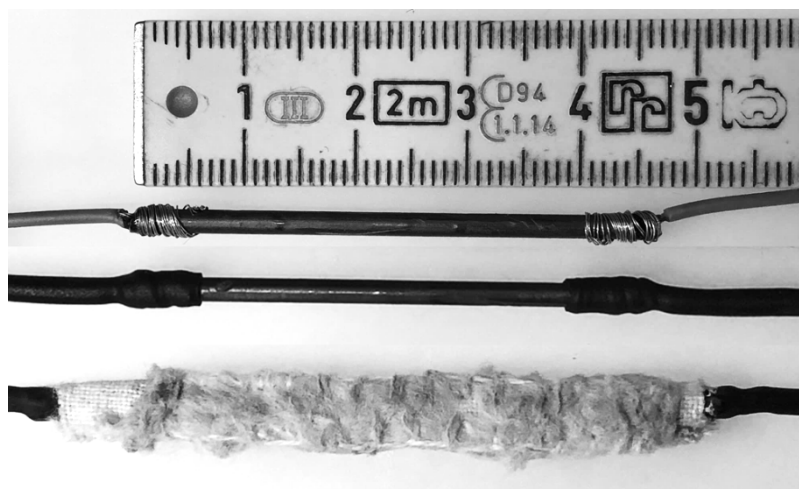
Fig.3: Three steps of constructing the plating tool based on pencil graphite as described above. In the bottom, a thin layer of cotton is additionally sewn to the fabric for the solution to easily also reach the waveguides inner corners.
