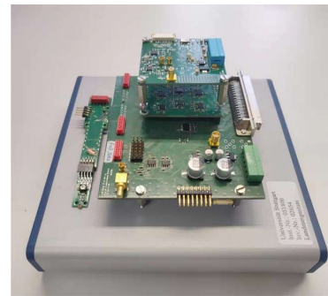
Figure 12. (a) Block diagram and (b) photograph of all electronics of the presented CMOS-based NMR platform
