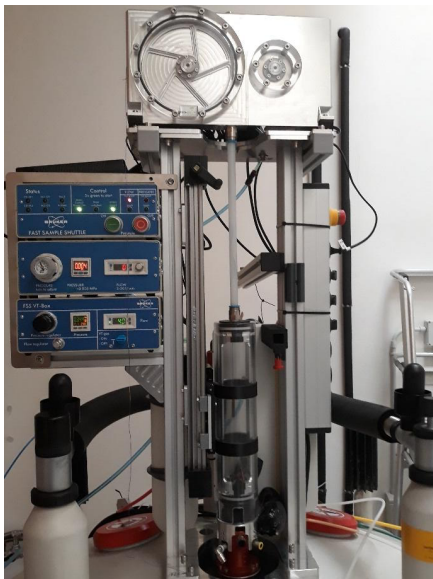
138 139 Figure 2. Photograph of the FSS installed on the 700 MHz NMR spectrometer at CERM in Florence, Italy.
